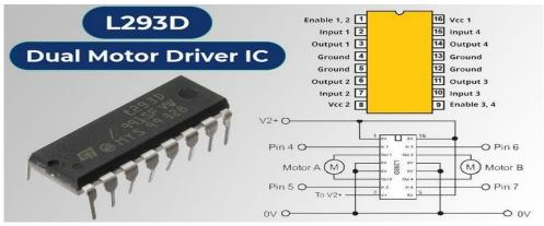
Fig 4: L293d Dual Motor Driver IC Pin Configuration
